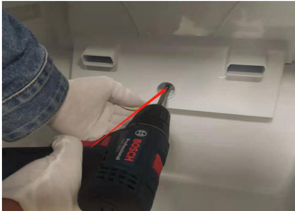
Step I: Use a screwdriver to remove the fixing screws of freezing air duct;
