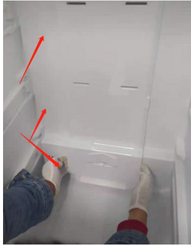
Step I: Disassemble the refrigerating air duct assembly from the top down
