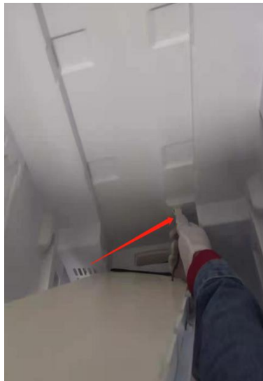
Step II: Disassemble the refrigerating air duct assembly from the refrigerator, as shown in the diagram, and unplug the connecting terminals
