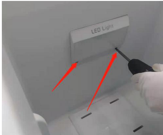
Step I: Remove the 2 screws at the rear of the assembly
