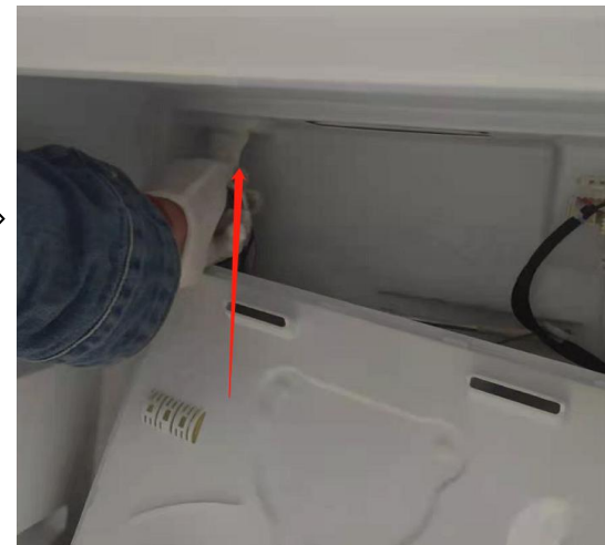
Step III: Unplug the freezing air duct terminal and take out the freezing air duct;
