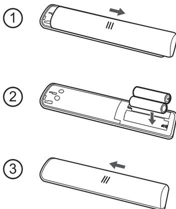
Insert batteries in the correct polarity as indicated in the battery compartment.
