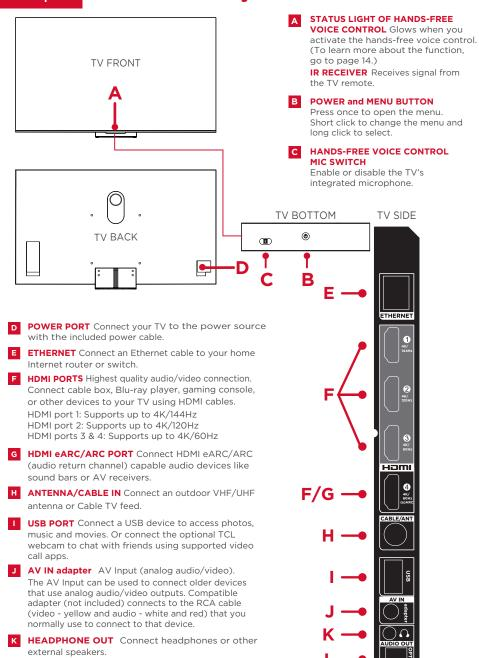
L OPTICAL (DIGITAL AUDIO OUT) Connect an optical cable to an external digital audio system.
