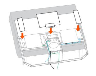
Put back the magnetic glass cover of the Subwoofer, and stick the footpads on the two ends of the bottom stand bracket.
