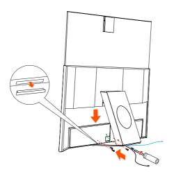
Plug the Sound Bar connection cable to the port on the Sound Bar. All installation is now completed.
