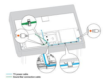
Put the two connectors at the bottom and get the Sound Bar connection cable and the TV power cable out through the left connector as illustrated. Then fix the two connectors with 6 M5X15mm screws.
