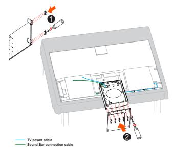
Plug in the Subwoofer power cable, and let the TV power cable and the Sound Bar connection cable go through the groove as illustrated.
