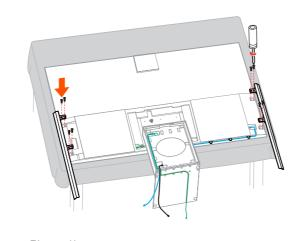
Secure the two ends of the bottom stand bracket to the left and right stand brackets with 6 M4X10 screws. Secure the middle part of the bottom stand bracket to the stand plate with 6 M3X6mm screws. Refer to the illustration
