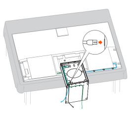
Align the left and right stand brackets on the back of the TV and secure them to the TV with 8 M5X15mm screws.
