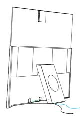
Peel the tape and film off the Sound Bar as illustrated, then stick the two footpads on the two ends of the bottom of the Sound Bar.
