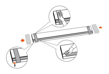
Remove the rubber plugs on the bottom of the Sound Bar, then match the Sound Bar with the linking plates and fix them with 4 M4X6mm screws.
