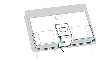
Plug in the Subwoofer power cable, and let the TV power cable and the Sound Bar connection cable go through the groove as illustrated.
