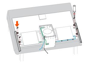
Peel the tape and film off the Sound Bar as illustrated, then match the Sound Bar with the stand plate and fix it with 4 M4X6mm screws.
