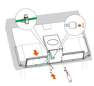
Secure the two ends of the bottom stand bracket to the left and right stand brackets with 6 M4X10mm screws. Secure the middle part of the bottom stand bracket to the stand plate with 5 M3X6mm screws. Refer to the illustration below.
