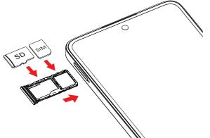
Place or remove the Nano SIM card and the microSD™ card in the correct slot as shown. Please note that gold contacts must be facing down.
