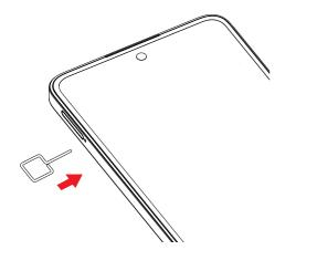
Locate the SIM tray located on the side of your device. Insert the provided SIM pin into the hole and pull out the SIM tray.
