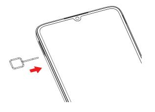
Locate the SIM tray located on the side of your device. Insert the provided SIM pin into the hole and pull out the SIM tray.
