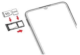
Place or remove the Nano SIM card and the microSD<sup>™</sup> card in the correct slot as shown. Please note that gold contacts must be facing down.
