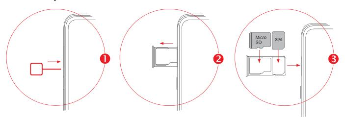
You must insert your SIM card to make phone calls. You do not need to power off your phone before inserting or removing the SIM card as this phone supports hot swap.
