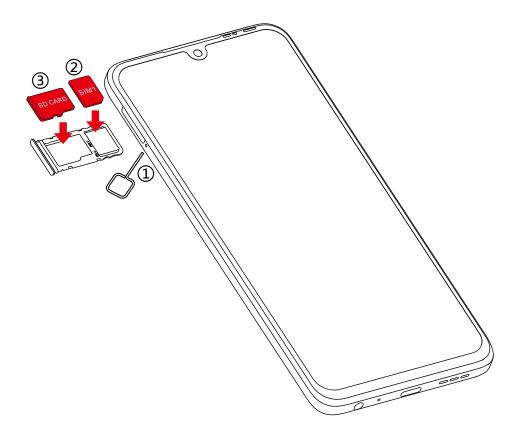
You must insert your SIM card to make phone calls. You do not need to power off your phone before inserting or removing the SIM card as this phone supports hot swap.
