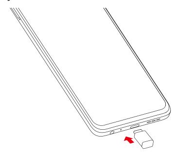
Your phone is partially charged. Charge the battery by using the USB-C cable and charger provided. You are advised to fully charge the battery ( ). Charging status is indicated by a percentage displayed on screen while the phone is powered off. The percentage increases as the phone is charged.
