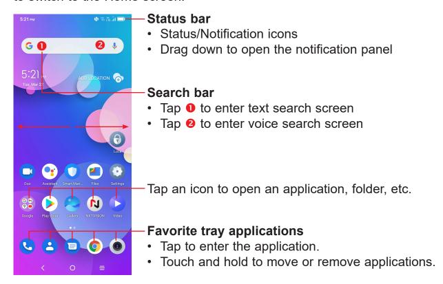
The Home screen is provided in an extended format to allow more space for adding applications, shortcuts etc. Slide the Home screen horizontally left and right to get a complete view.
