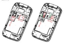
To remove the SIM card or microSD card, press down on the small plastic tab (0), then slide out the card (2). Do not use force or any sharp objects.
