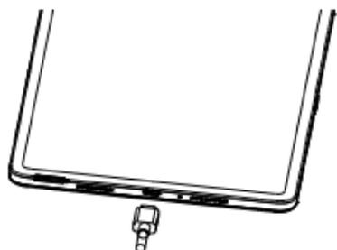
1. Insert the USB Type-C cable into the charge port as shown.
