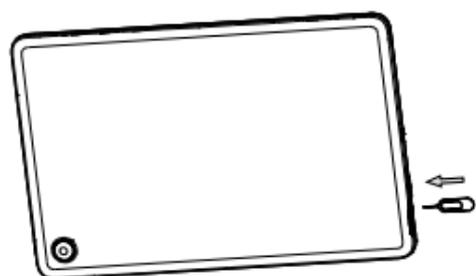
Insert the SIM pin that's provided to eject the SIM tray and then slide it out gently.
