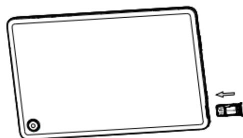
Place or remove the Nano SIM card and the microSD™ card in the correct slot as shown.
