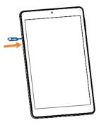
**Step 2.** Remove the NANO SIM card/microSD card tray.
