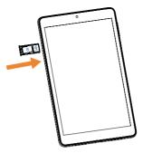
**Step 4.** Slide the tray slowly into the SIM tray slot. It only fits one direction. Do not force into place. Keep the SIM tool in a safe place for future use.
