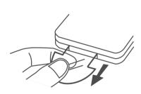
4b Replace the remote control battery
